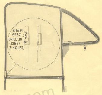
Remove the window runway and ventilating window from the door. Drill two No. 30 drill size holes so that extension can be installed. The lower end of the extension should be ½ inch from the bottom of the cross bar which is spot welded holding the two sides of frame together.
