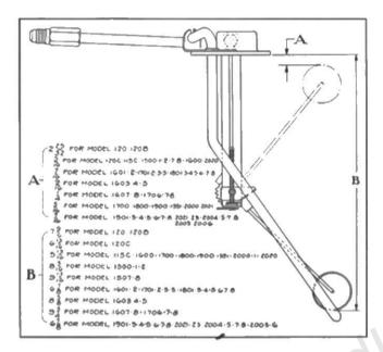
Before making the installation of a tank unit, it is necessary that the cork float at the bottom of the wire arm be properly located in order that a correct reading may be shown, and this illustration indicates the distance from the top of the tank to both the top and the bottom of the float.
