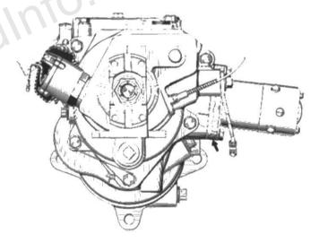
The trouble proved to be the position in which the metal spacer between the solenoid and the Econo-Drive housing was installed. The center hole in this spacer through which the solenoid shaft passes is offset. Although the two attaching cap screw holes will line up in either position, there is only one way to install the spacer so that the shaft will clear the hole in the spacer.
