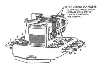
A quick check of the relay may be made by holding the points on the upper coil closed with your finger. This will cause the lower points to close.
