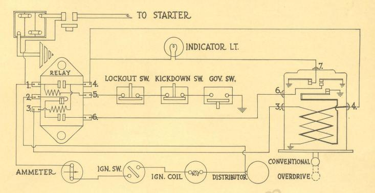
This diagram shows the electrical circuits of the overdrive mechanism.
