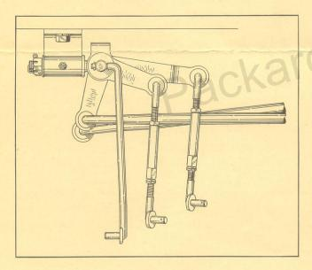
When excessive lost motion develops in the gear shift linkage it may be found that no one point is responsible. It is more likely to be the accumulated clearances at all the wearing points.
