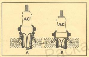
Insulator (A) is longer, therefore will run "hotter." Insulator (B) is shorter, therefore will run "cooler."
