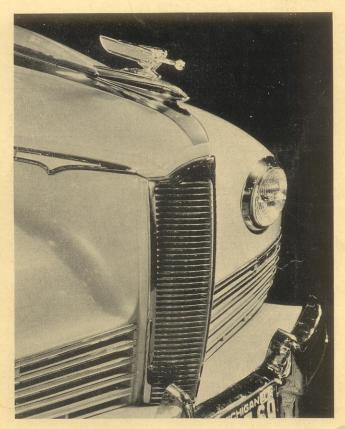
DeLuxe emblems with crystal wings may be installed on Clipper models. The drawing gives the necessary information and the photograph shows the pleasing result.
