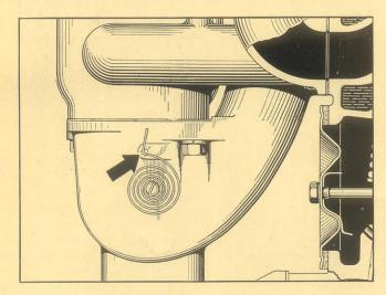
If the heat valve sticks in the cold position with the weight up, the gas passes through the hot spot at all times. This will develop too much heat in warm weather. It will cause the ragged operation of the motor and may even develop vapor lock.
