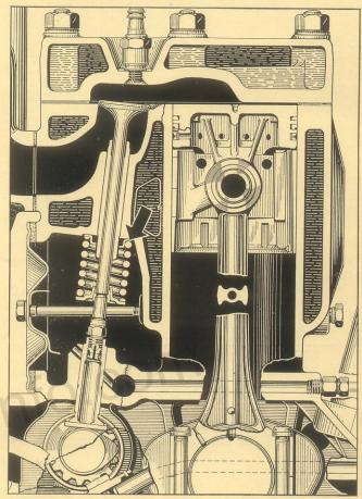
In those cases where the original construction includes a collar type washer or a Shakeproof washer, one Shakeproof can be added, but care must be taken not to build up the washer thickness any further. The upper end of the spring is centered by the recess in the cylinder block, and the recess must not be filled with washers to the point where it can no longer locate the spring.
