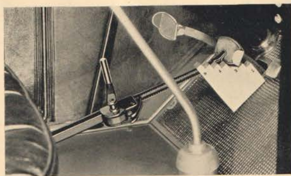
Figure Four The brake pedal depressed. Pedal depressor S. T. 190 holding the pedal against Pedal Depression gauge S. T. 659.
