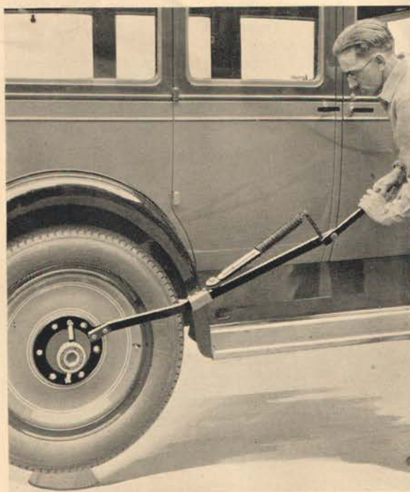
Figure Five Brake testing scale S. T. 658 (S. T. 673 for 5th Series) attached to the wheel. Scale should read 90 lbs. front, 100 lbs. rear.
