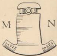
FIGURE TWO S. T. 682 Synchronizing Tool for use on 526-533 distributors.
