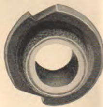
FIGURE FIVE S. T. 685 Breaker gauge for use on the 443 distributor.
