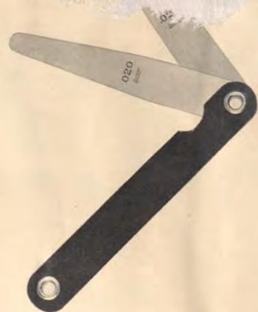
FIGURE FOUR S. T. 657 a handy thickness gauge in a fibre case. It has two blades, one .020" for the distributor breaker gap, and one .025" for the spark plug gap.
