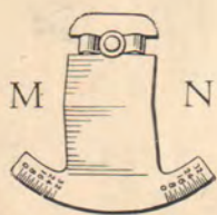
FIGURE TWO S. T. 682 Synchronizing Tool for use on 526-533 distributors.
