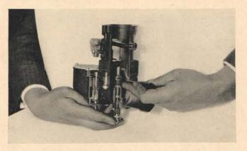
Remove deflector from air intake. Run finger into air opening and hold it against the metering head, then turn adjusting handle on metering pin until the pin seats, which will be noted when the metering head is reached and an upward pressure is felt against the finger in the air intake.
