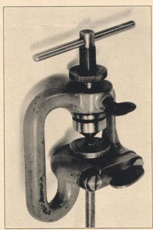
The flaring tool will accommodate four different sizes of tubing  $\frac{3}{16}$ ",  $\frac{1}{4}$ ",  $\frac{5}{16}$ " or  $\frac{3}{8}$ ". This tool is designed to flare the end of the tube with spinning action so that tubing will not crack or split at the flare.
