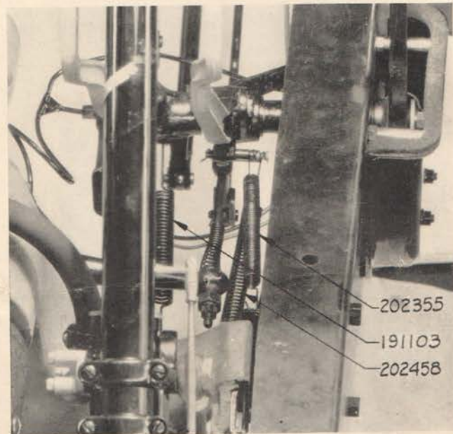
CORRECT LOCATION OF RETRACTING SPRINGS
