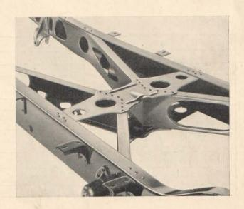
point; reinforced rear end structures and improved method of fastening body to frame; improved weight distribution, improved balance of spring and shock absorber rates—all contribute to a new degree of solidity and a characteristic softness in the ride by eliminating road "harshness."
