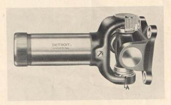
On the new type universal joint an inspection should be made on all cars which left the factory prior to October 3, 1934 to determine the condition of the spring lock (A) which holds the spider bearing in place. In the event any of these are found broken, or loose a new one—piece No. 22557 should be installed.
