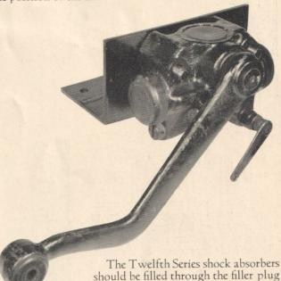
and never by removing the end The filler plug permits a slight amount of air to remain in the top of the shock absorber in order to take care of expansion through heat, and thus prevent the damage which may follow if the shock absorber is
