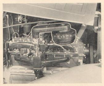
The Heavy Duty Air Cleaner actually has THREE stages of cleaning—(1) Reversal of intake air through the louvre openings (2) Cleaning of air in the Oil Bath
