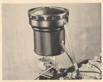
Actually, it is very difficult to prescribe the intervals at which cleaning is necessary since this depends not on miles driven or days of operation, but solely on the amount of dust filtered out of the air by the cleaner.
