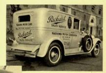
You will notice a rear door replaces the worst part of the damaged body. Also the rear quarter glass and rear door glass were replaced with a sheet steel panel. The interior of the car being replaced with a board flooring and 1/4-inch board side panels, and a
