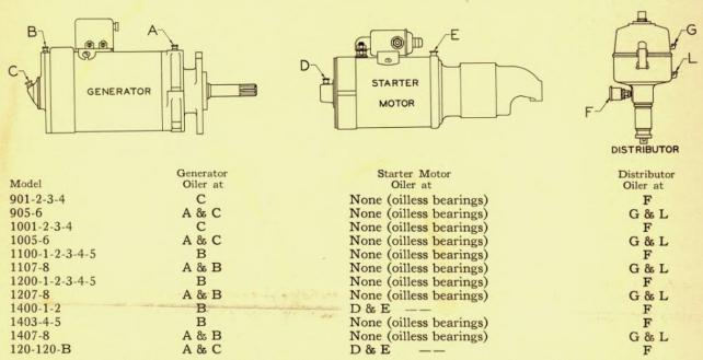
A few drops of engine oil every 2000 miles in the oilers of generator, starter motor or distributor. Turn down grease cup on distributor shaft every 2000 miles and refill if necessary. Use No. 3 cup grease.
