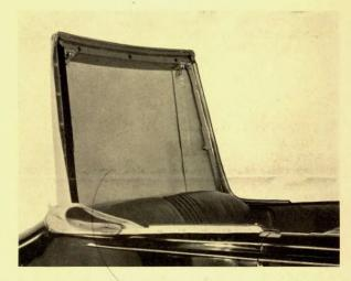
2. In order to gain additional space in the top compartment at the back of the rear seat, the seat cushion should, by means of the handle provided, be raised off the dowel pins. Hold the cushion off the pins and pull the seat back as far forward as possible. This will give the space required for holding the top when folded.
