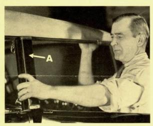
4. Unfasten center post header clamp at top of post, unscrew clamp at bottom of post, and by slightly raising top at windshield, to relieve tension, remove center posts A. Storage space for the posts will be found in the compartment underneath the driver's seat, the door of which is at the bottom of the seat back.
