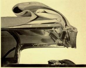
9. Make sure that the front clamps, which hold the top to the windshield, are in the *up* position. By pushing the front cross piece backward, fold the bows back and fold the material smoothly back on the top.
