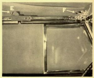
7. Release two thumb screws E at front rail joints just forward of pillar post joints.
