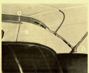
5. Unfasten zippers on both sides of back curtains B.6. Release plunger type catches C at top of curtain and drop to outside.
