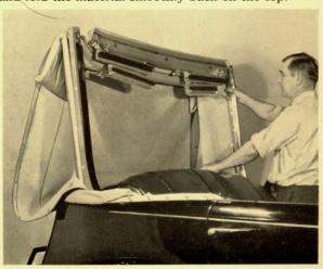
10. Tip the top backward into an upright position, folding the pads into the inside of the top compartment. Allow the top material to drop back on to the outside.
