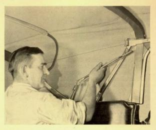
1. Instead of lever clamps at the rear prop irons, header bar supports are used. These are released and folded into the side compartments.
