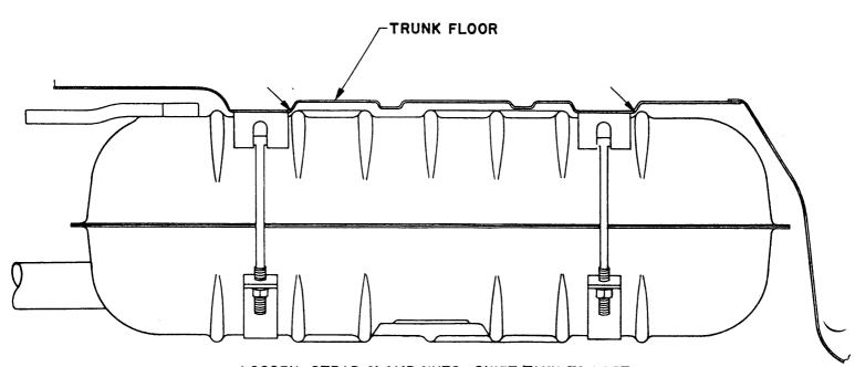
LOOSEN STRAP CLAMP NUTS - SHIFT TANK TO LEFT AS FAR AS POSSIBLE AS INDICATED BY ARROWS.
