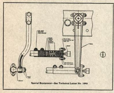
We have developed a ball and socket joint which may be used to replace the block and pin joint at the rear end of the steering connecting rod on first and second series Twin-Six cars.
