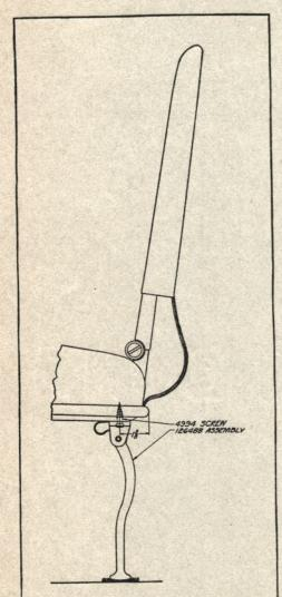
An extra support for the Packard Six Coupe folding seat has been developed which may be applied to any vehicle now in service.
