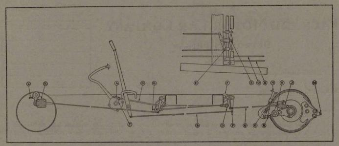
With all above adjustments made, the foot brake should start to hold after about 2" of pedal travel and the rear wheels should slide on dry pavement when the pedal pad is about 1" from toe board.
