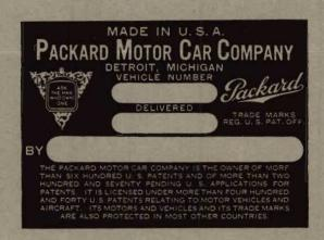
The illustration shows the Patent Plate which is mounted on the dash of all Packard cars. It is attached to the forward side of the dash and is in a very accessible position.
