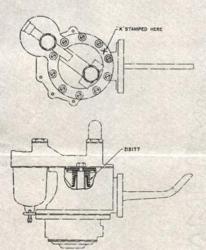
A motor miss which occurs at high speeds may be due to the fact that the fuel pump is not delivering a sufficient supply of gasoline to the carburetor.
