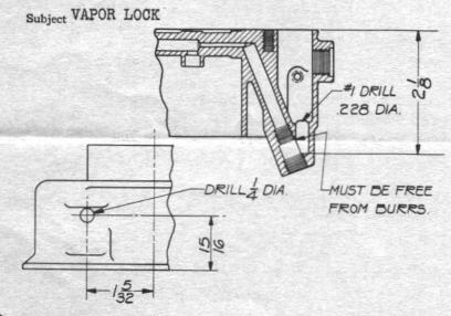
The terms vapor lock and percolation are generally used to describe the vaporizing of the fuel before it has passed through the carburetor.
