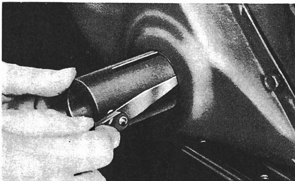
Fig. 33—The Gear Cover Should Be Shifted to Obtain the Same Clearance Around all Sides of the Arbor.
