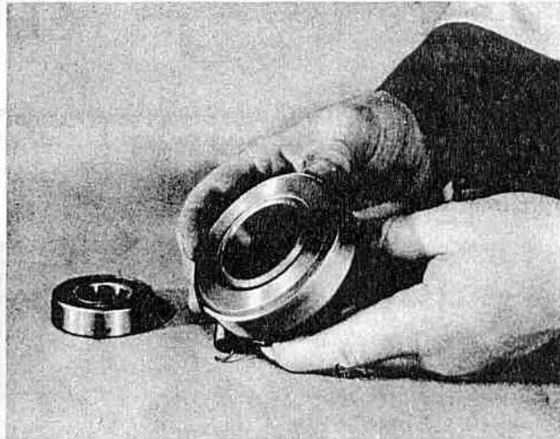
Figure 5—Inspecting the Clutch Release Bearing
