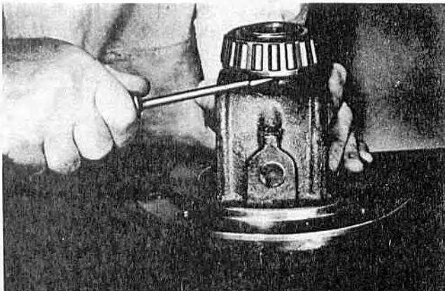
Figure 12—Checking the Fit of the Differential Case Side Bearings
