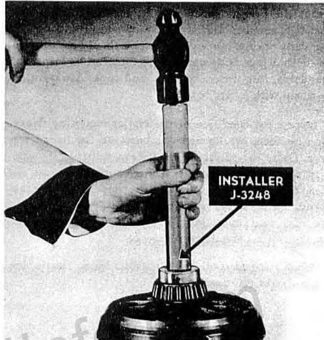
Figure 17—Installing the Differential Side Bearing
