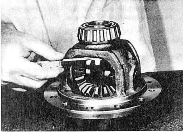
Figure 19—Measuring the End Play of the Differential Side Gears
