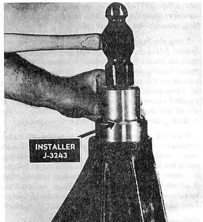
Figure 15—Installing the Pinion Front Bearing Cup
