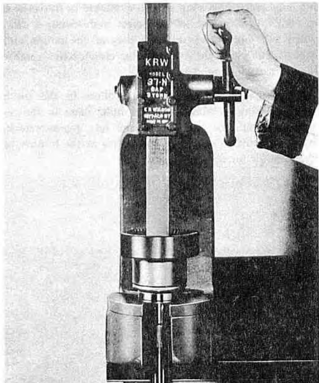
Figure 48—Pressing On the Overdrive Main Shaft Rear Bearing
