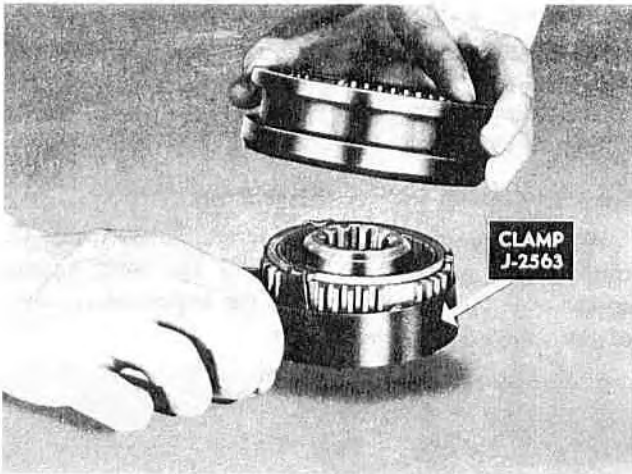
Figure 32—Assembling the Synchronizing Unit
