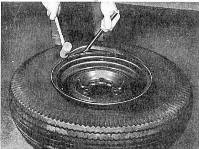
Figure 3—Installing the Tire on the Wheel
