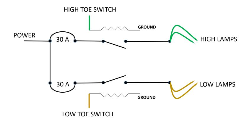
Colored wires represent existing headlight wiring. Black segments represent new wiring and/or components.
