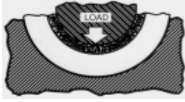
ENGINE BEARINGS RIDE ON A FILM OF OIL
